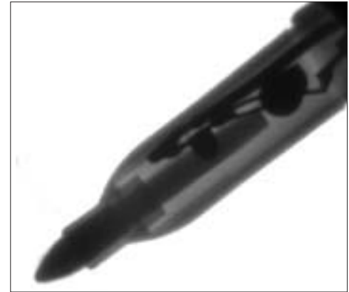
Electronics concealed inside a pen
